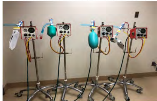
Figure 1B: Four Percussionaire™ pneumatic-driven ventilators shown ventilating a variety of surrogate lungs.
