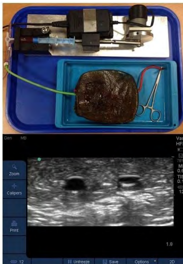
[Figure 1. Top: Motorised arterial simulation pump connected to artery analogue in ADAM gel. Bottom: Static ultrasound image taken at the end of the study to show artery with pump driven pulsation (left) and adjacent compressible vein (right) to enable arterial cannulation]
